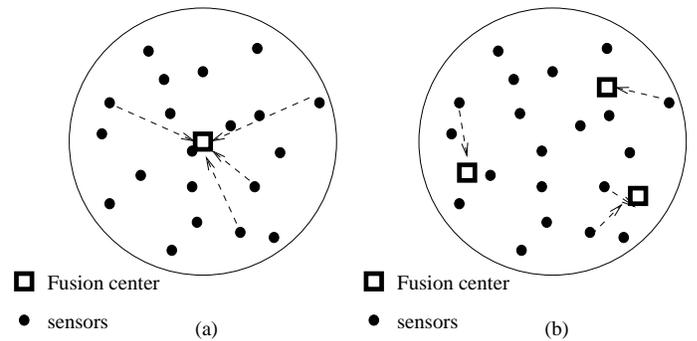
Fig. 1. WSNs: (a) the first type where there is one FC; (b) the second type where there are multiple LFCs.
