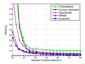
Fig. 6. Comparison of average worst case error for the same experimental setup as Fig. 5. We explicitly show the WCE lower bound value  $\alpha^{-1}=0.01$ .
