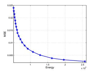
Fig. 10. Pareto curve of energy consumption versus MSE levels obtained by (20) with  $\lambda = 10^3$  over T = 10 time instances for a fixed sensor network of m = 100 elements that estimate an unknown of size n = 20. The network topology we consider is shown in Fig. 1.
