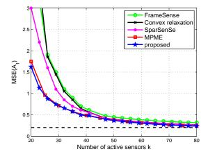
Fig. 5. Comparison of average mean squared error for the estimation of a variable of size n=20 with a sensor network of m=100 sensors. The measurement matrix is a random  $\alpha$ -tight with  $\alpha=100$  and the results are averaged over 100 realizations. We explicitly show the MSE lower bound value  $n\alpha^{-1}=0.2$ .
