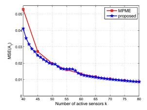
Fig. 3. Average mean squared error reached by MPME [4] and the proposed method for the estimation of a variable of size n=40 with a sensor network of maximum m=100 elements. The measurement matrix is random Gaussian and the results shown are averaged over 100 realizations.
