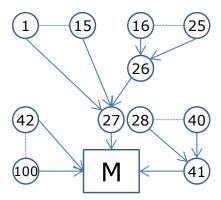
Fig. 1. An example of network topology consisting of m=100 sensors and a master node M. In the scenarios we consider each sensor has a dual role: it can perform a linear measurement and/or forward data from other sensors. To avoid routing issues, we consider a single (possible multi-hop) predefined path from each sensor to the master.
