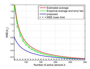
Fig. 2. Expected versus empirical values of  $MSE(\mathbf{A}_1)$  constructed by selecting k sensors from a total of m belonging to random tight frame  $\mathbf{A} \in \mathbb{R}^{m \times n}$  with  $\alpha = m = 300$  and n = 40. Empirical results are averaged over  $10^5$  random sensor selections from  $\mathbf{A}$ . We show the lower limit of  $MSE(\mathbf{A}_1)$  which is  $MSE(\mathbf{A}) = nm^{-1}$  by (6) and is achieved by  $\mathbf{A}_1$  when k = m.
