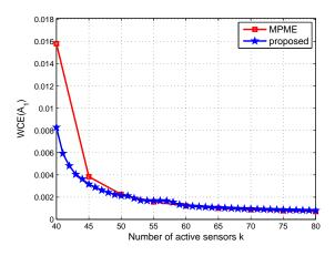
Fig. 4. Average worst case error reached by MPME [4] and the proposed method for the same experimental setup as Fig. 3.
