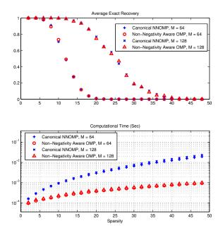
Fig. 2. Exact recovery (top panel) and computation time (botom panel). N = 256 and M = 64 & 128 are fixed while sparsity K is changing.
