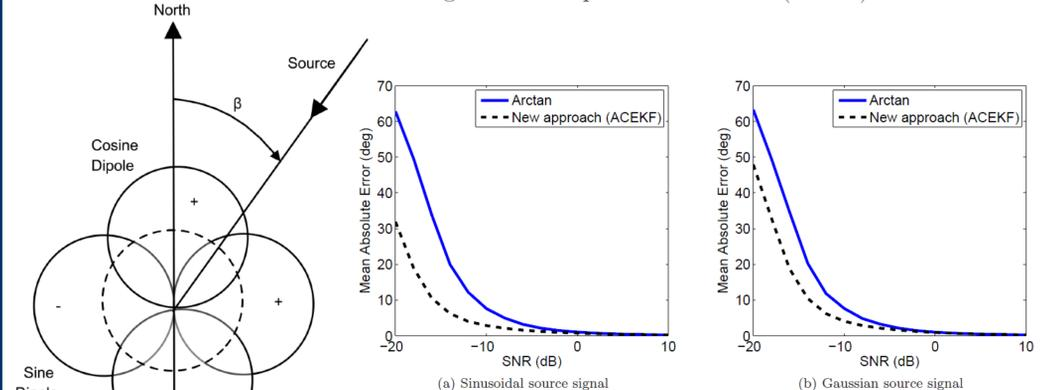
Performance comparison between the proposed widely linear approach and the standard arctan estimator
