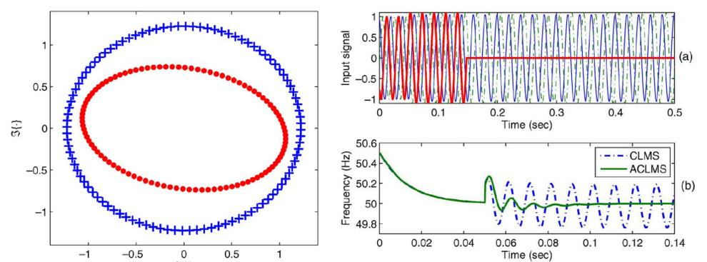
Frequency estimation in unbalanced Three-phase power systems using the widely linear (augmented) complex LMS (ACLMS) Algorithm
