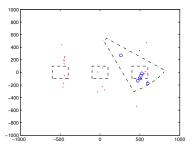
Fig. 1: Example of scenario. The focus regions are denoted by dotted rectangles, and the current field of view is denoted by a dotted triangle. The targets are red dots, and the current detections are blue circles.
