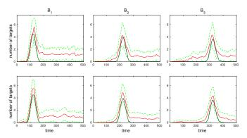
Fig. 4: Estimated target activity for naive (top) and variance-based (bottom) controllers ( $p_{\rm d}=0.8,\,\lambda_{\rm fa}=10$ ). True target number is in black, mean target number is in red, +/- standard deviation is in green.
