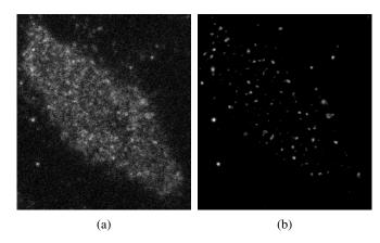
Fig. 1: Output of the à trous wavelet method on an example image acquired using STORM. Fig. 1a shows the noisy input image and Fig. 1b demonstrates the respective performance of the filter.
