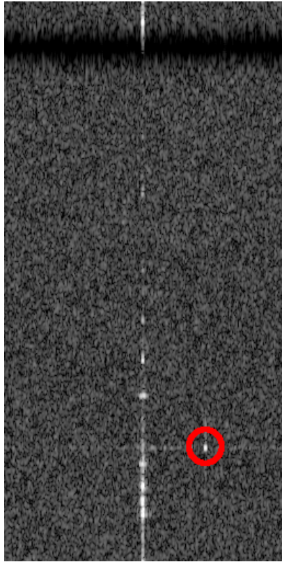
Fig. 6. Detection highlighted on range/Doppler map [12].
