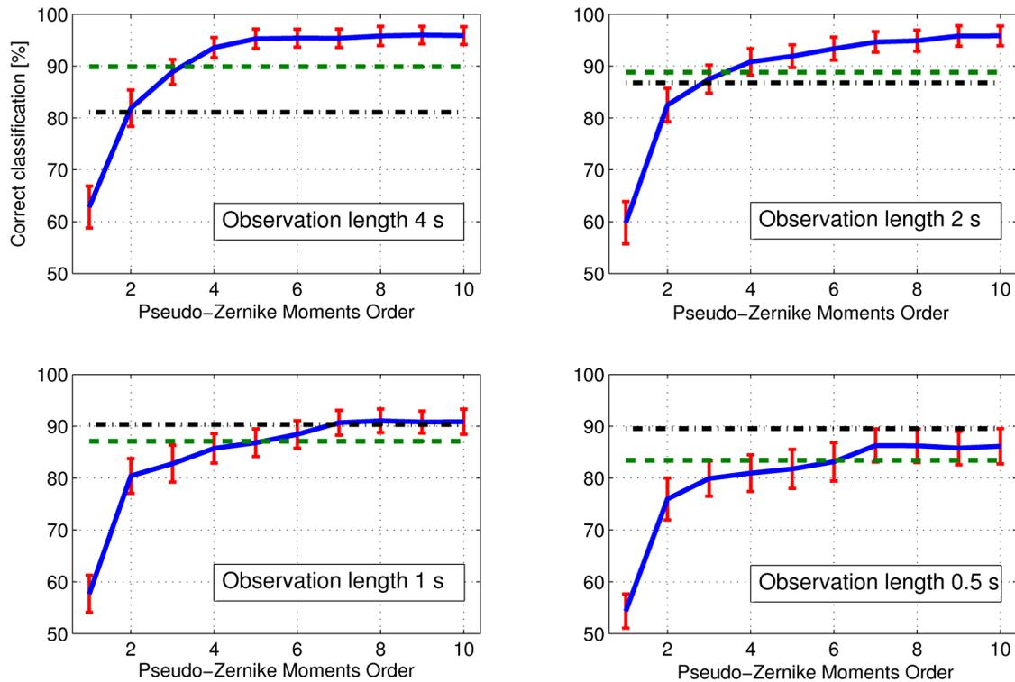
Fig. 3. Correct classification (%) versus pseudo-Zernike moments order. The solid line represents the average correct classification (over 50 runs) with its corresponding degree of reliability, the dashed curve is related to the MFP-based classifier proposed in [8], whereas the dot-dashed curve refers to the TFD-DF classifier given in [7]. Subplots refer to different signal lengths (i.e. 4, 2, 1 and 0.5 s, respectively).
