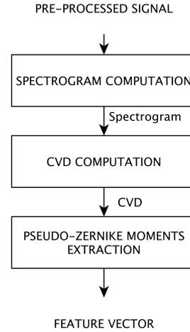
Fig. 1. Block scheme of the proposed feature extraction algorithm.
