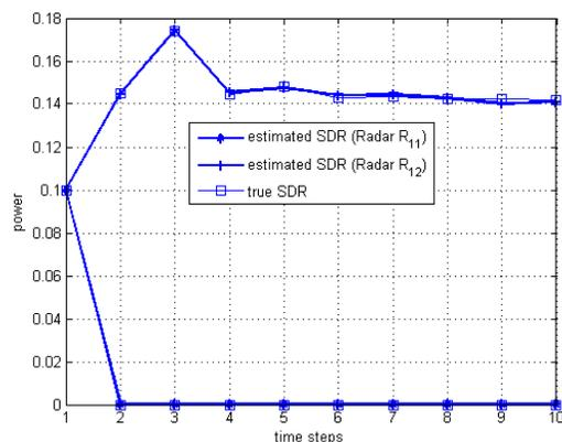
Fig. 9. The power allocated to radars by the game theoretic method using the true value and the estimated value of SDR ( $N = 512$ ) in the first cluster when  $K = 3$  and  $M = 2$ .
