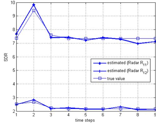
Fig. 4. The SDR values achieved by the game theoretic method using the true value and the estimated value of SDR ( $N = 64$ ) for the radars in the first cluster. The target SDR is 2.1599.
