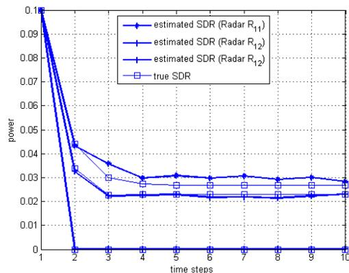
Fig. 8. The power allocated to radars by the game theoretic method using the true value and the estimated value of SDR ( $N = 64$ ) in the first cluster when  $K = 2$  and  $M = 3$ .
