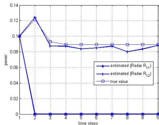
Fig. 6. The power allocated to radars by the game theoretic method using the true value and the estimated value of SDR ( $N = 64$ ) in the first cluster.
