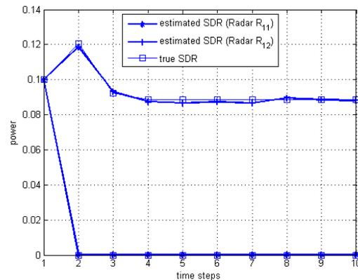
Fig. 5. The power allocated to radars by the game theoretic method using the true value and the estimated value of SDR ( $N = 512$ ) in the first cluster.
