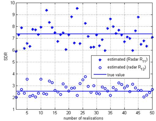
Fig. 2. Estimated and true values of SDR for a fixed transmission power  $p_{11} = p_{12} = 0.1W$  and  $N = 64$ .
