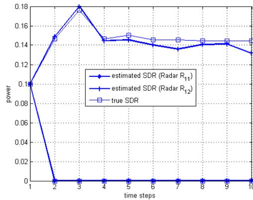
Fig. 10. The power allocated to radars by the game theoretic method using the true value and the estimated value of SDR ( $N = 64$ ) in the first cluster when  $K = 3$  and  $M = 2$ .
