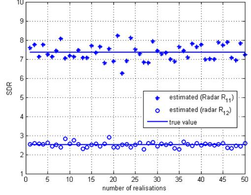
Fig. 1. Estimated and true values of SDR for a fixed transmission power  $p_{11} = p_{12} = 0.1W$  and  $N = 512$ .
