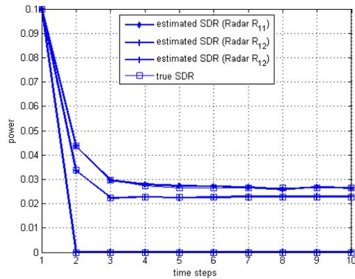
Fig. 7. The power allocated to radars by the game theoretic method using the true value and the estimated value of SDR ( $N = 512$ ) in the first cluster when  $K = 2$  and  $M = 3$ .
