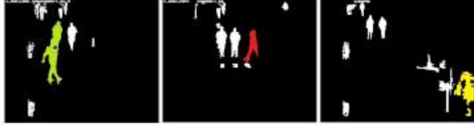
Figure 4.2. Examples of background subtraction results from the ‘EnterExitCrossingPaths1cor’ sequence of the CAVIAR dataset. The left, middle and right figures correspond to frame 188, 67 and 345 respectively. The green part in the left figure shows the occlusion of two human targets, which may cause missed detection; the red part in the middle figure shows the appearance of another human target and the yellow part in the right figure shows the disappearance of a human target. Noise components can be observed in the background subtraction results, including patches of salt and pepper noise, which may cause false alarms in the multiple human tracking.
