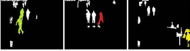
**Fig. 1:** Background subtraction results for three frames in the sequence from CAVIAR dataset, where the green part in the first figure shows the occlusion of two human targets; the red part in the second figure shows the appearance of another human target and the yellow part in the third figure shows the disappearance of a human target.
