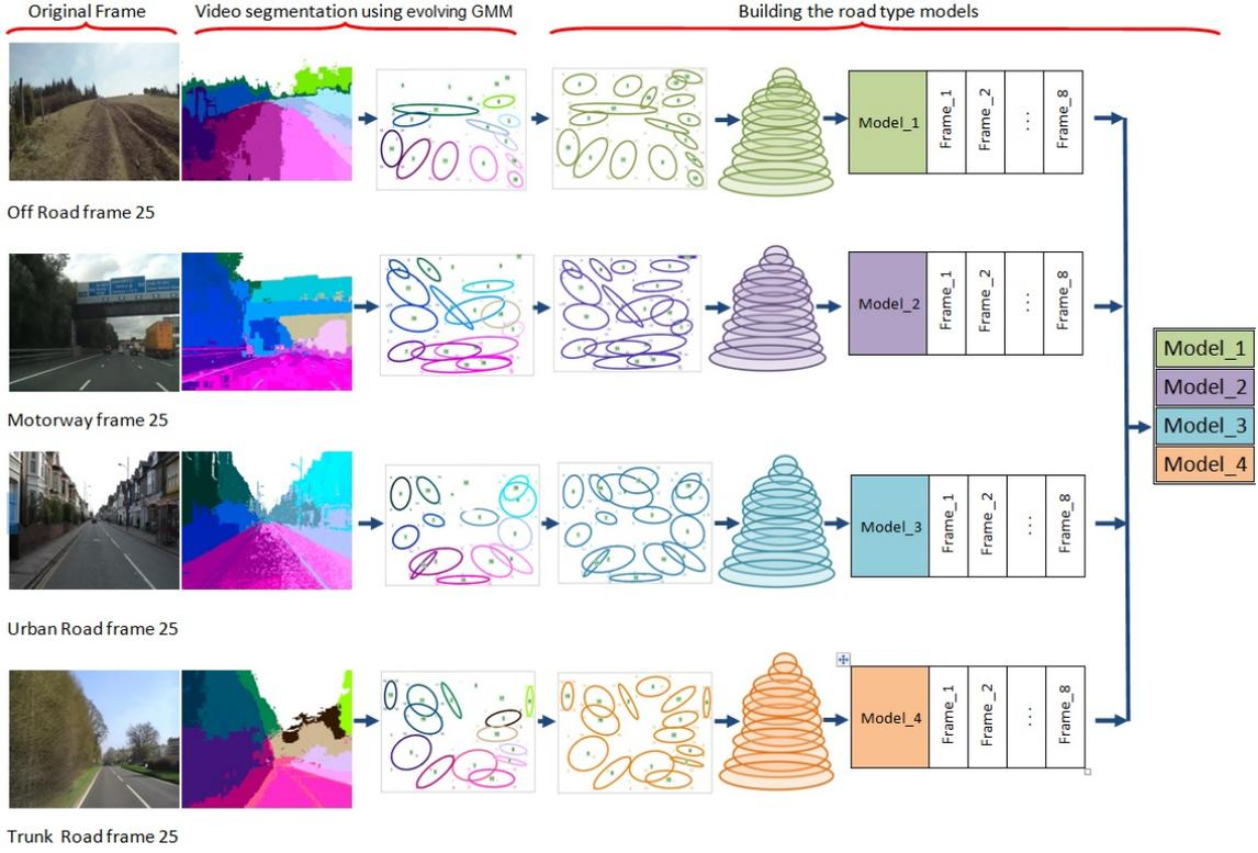
Fig. 1. The process of building the road-type models.
