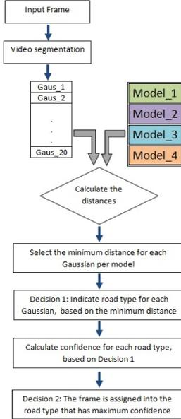
Fig. 2. The pipeline of the classification process.
